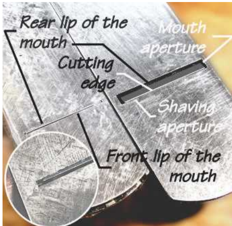
▲ Pic. 5 The mouth aperture of a block plane (left) differs a lot from that of a smoothing plane
